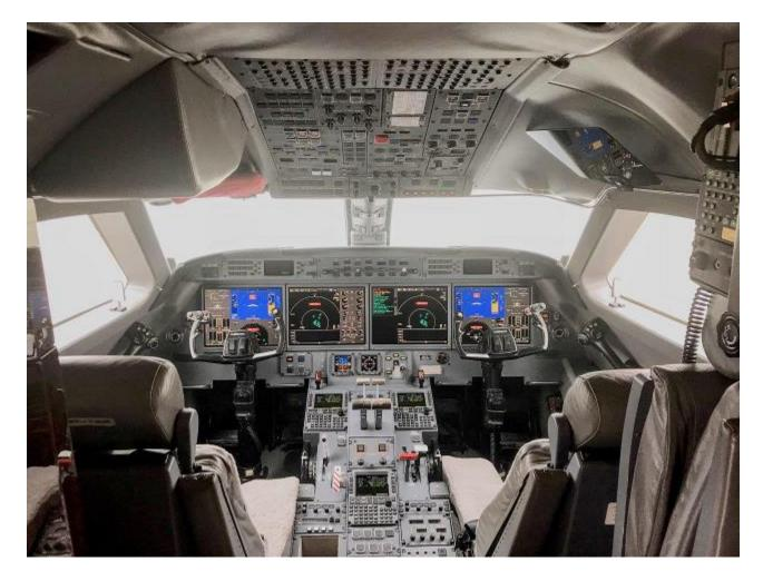
AVIONICS: Enrolled on Honeywell Avionics Protection Plan Autopilot: Dual Honeywell GP-500 Air Data Computers: Dual Honeywell MC-850 COMM w/SELCAL: Dual Collins HF-9000 DME: Dual Honeywell DM-855 ELT: Artex 110-C406 FMS: Triple Honeywell HF COM: Dual Collins HF-9000 IRS: Triple Honeywell IR-500 Laseref V Radar ALT: Dual Honeywell RT-300 TCAS L3 RT-951 w/ Change 7.1 WX Satellite Weather: Dual Honeywell Primus 880
